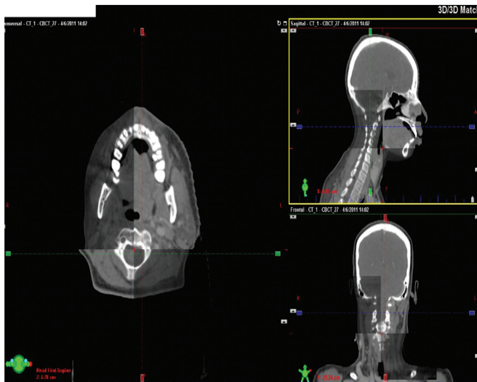
Figure 3. Modified Image-guided Radiation Therapy (IGRT), and anatomy match performed on CBCT image fused to planning CT.
